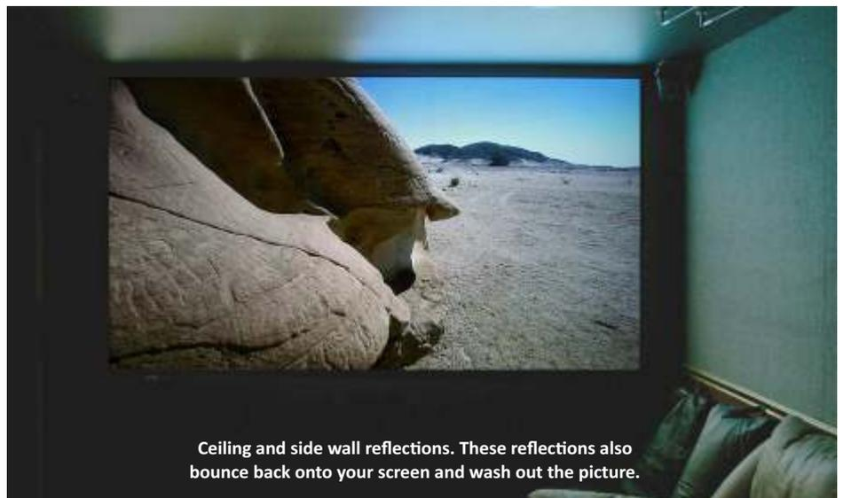
Ceiling and side wall reflections. These reflections also bounce back onto your screen and wash out the picture.
