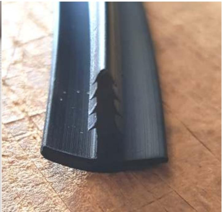
Above our brilliant new fabric insert profile. This is a 100 series PVC extrusion with 4 sets of flexible wings. A breeze to insert, easy to remove yet hard to push out under tension. Based on the snap buttons used in the automotive industry.
